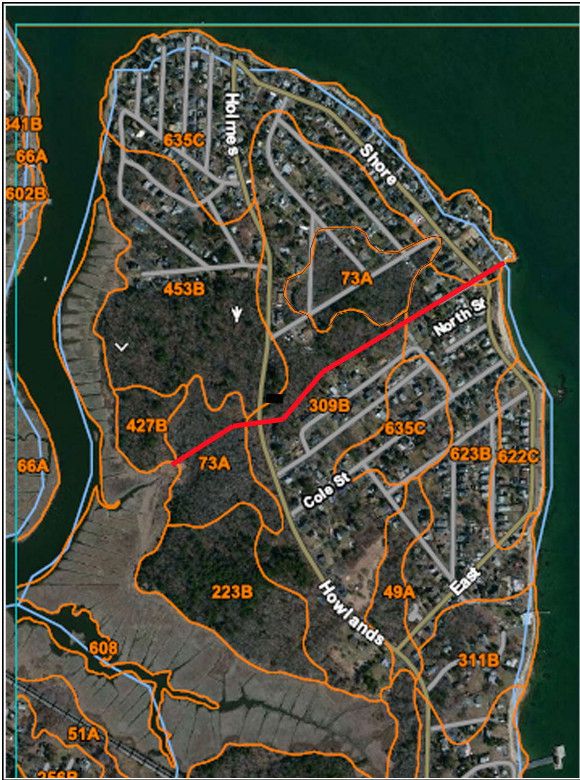
Figure 1. Soils within John Howland's bounds on Rocky Nook (Red line is the Howland Cooke boundary; Black rectangle is the Howland House) 73A: Whitman Loam; 309B: Moshup Loam 427B: Newfields Fine Sandy Loam; 453B: Gloucester-Canton Complex; 623B: Woodbridge Scituate Urban; 635C: Canton Urban
